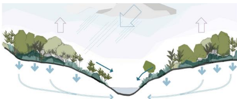
Figure 4: The water cycle interacts with plant and soil systems that capture, infiltrate and transpire rainwater and stormwater runoff.
