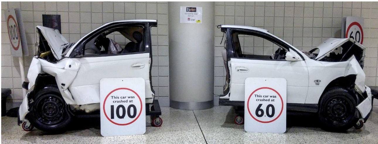
Figure 2.5: Difference in deformation striking a solid object at 60 and 100 km/h
